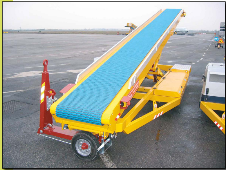
LUGGAGE HANDLING BELT WITH MODULAR BELTS WITH RUBBER INSERTS.
