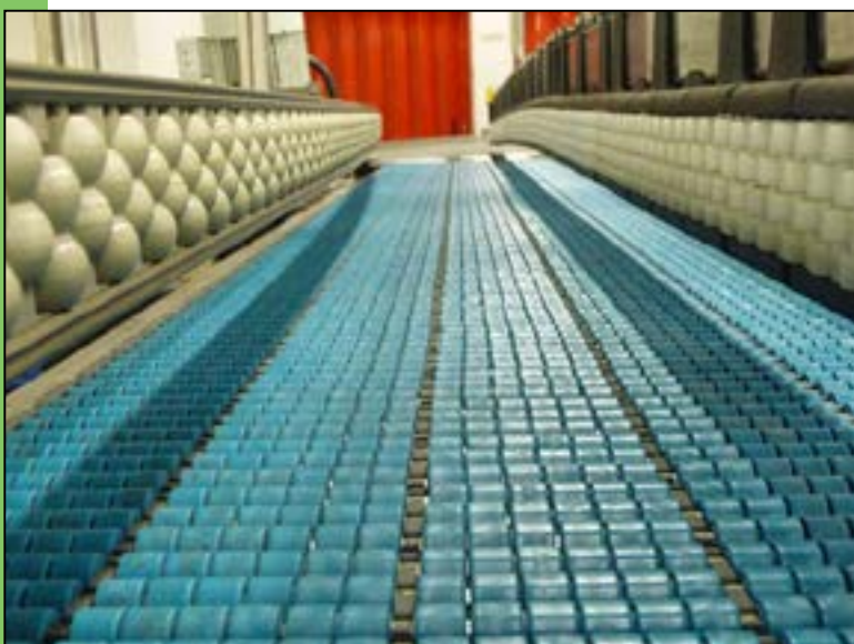
ACCUMULATION SYSTEM FOR SHRINK WRAPPED PRODUCTS.
